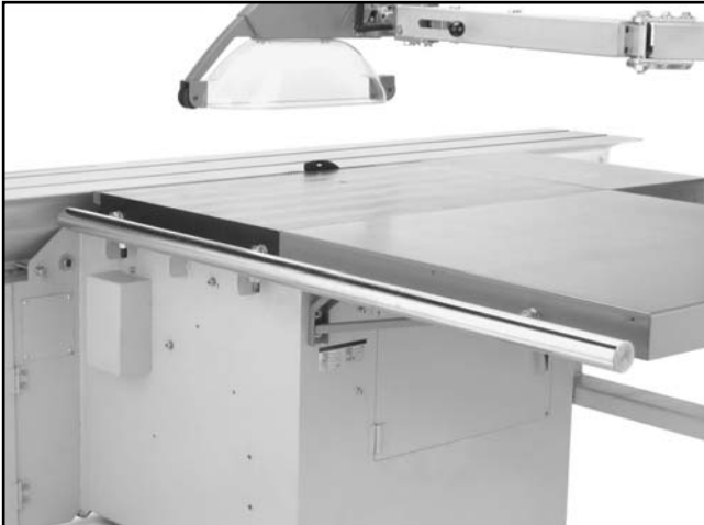
Figure 42. Fence rail installed.
